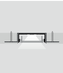
Incasso con cassaforma Recessed with formwork
